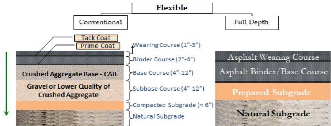
Figure 8 Cross-Sectional View of Flexible Pavements
