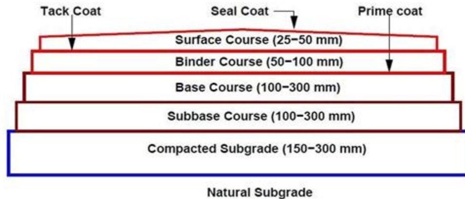
Figure 64 Typical Layers of a Flexible Pavement
