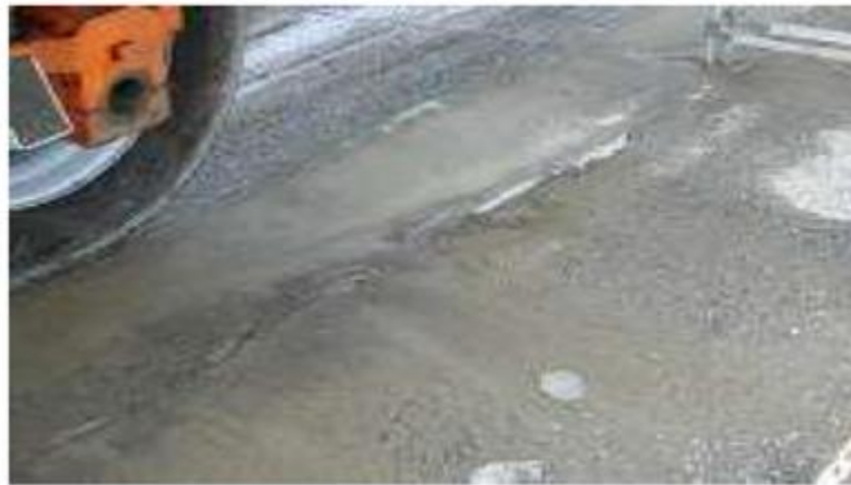
Figure 82 Pumping Evidence during High Vehicle Simulator (HVS) Test
